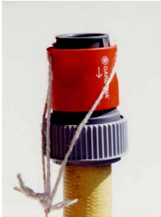
This is the garden hose fitting with the string attached to it. It is in the release position (the orange plastic piece is being pulled down).
