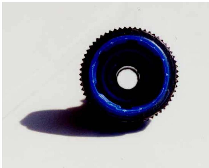
This is one end of the garden hose fitting, with a bottle cap glued in to make the nozzle.
