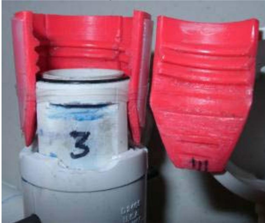
The four red collet pieces were originally a [Tornado Tube®](#)—my Dremel tool brought about the transformation. With the trigger ring in place, the force of the pressurized bottle cannot pull the collet pieces out of the head unit, due to mutually opposing ledges between the “bare” head and collet pieces.
