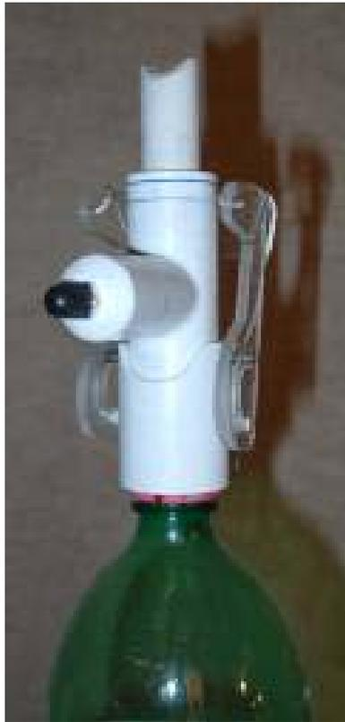
The assembled head unit is easily removed from the base. This allows the head to be attached to an inverted rocket, so that water does not spill out. Basically, the bottle screws onto the head just like one would install a light bulb in a socket. Nothing could be quicker or easier.
