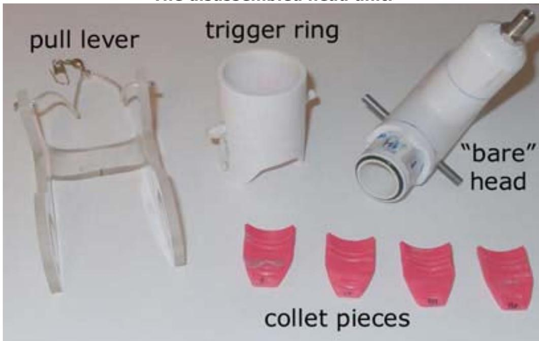
The pull lever is made of acrylic, which can be shaped when heated. The trigger ring and "bare" head units are made mostly of PVC plumbing parts. The head is pressure-tight and seals against the bottom of the bottle with an o-ring. I used a lathe to cut a precision groove for the o-ring. A Shraeder valve on the head allows pressurized gas to be added to the rocket.
